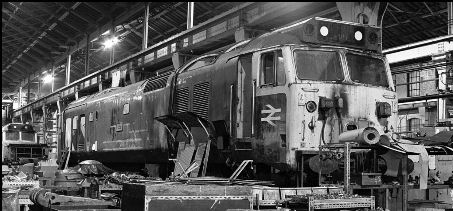
Above: Workshop photography has always been an interesting subject and in the days when access was easier to such establishments some unusual illustrations could be recorded. On 10 December 1979, Class 50 No. 50027 Lion poses in the main erecting shop at BREL Doncaster Works during an intermediate overhaul. This was the period in which Class 50 overhauls were being transferred from Crewe to Doncaster Works. Colin J. Marsden Photographic details: Camera: Mamiya 645 1000S, Lens: Mamiya 80mm, TriX at 400ASA, Exposure: 10sec @ f56. Negative scanned on Nikon Coolscan9000 at 600dpi.
