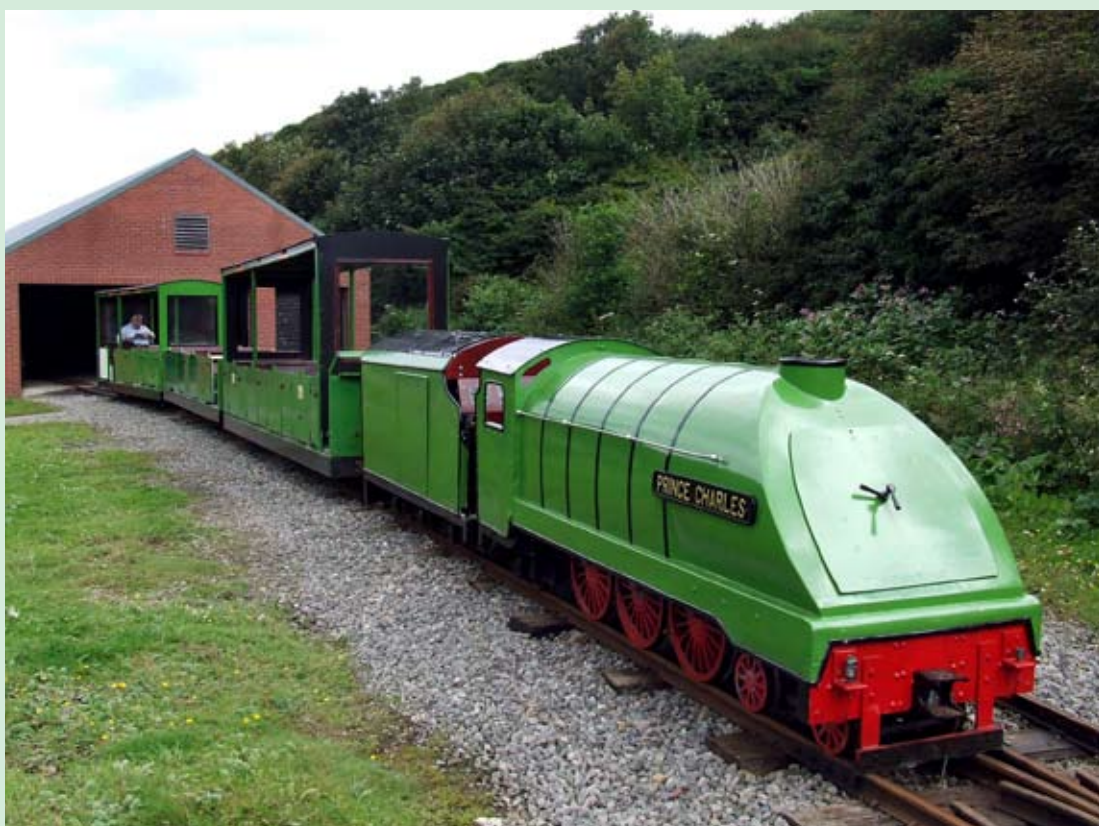
Right: This year marks the Diamond Jubilee of the Saltburn Miniature Railway, operated in Saltburn Valley Gardens. The 15in gauge line boasts two locomotives Prince Charles and George Outhwaite, four passenger carriages and various trucks. The locomotive Prince Charles, although to an 'A4' outline is a Diesel - Electric, 4-6-2, built around 1950 by the late H. Barlow. This locomotive was one of eight similar locomotives, built by Barlow, during the 1950s, six still remain. The loco is seen 'on shed' coupled to its passenger train on 8 July 2007.
