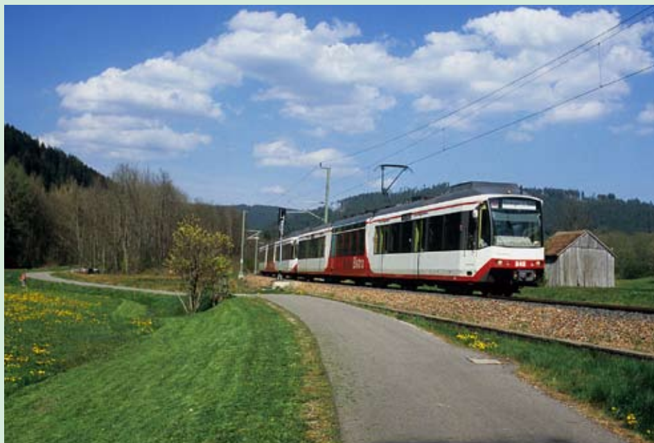
Left: Many regional lines in Southwest Germany are now served by the 'train-tram' units of the Duewag GT8-100 class owned by the regional carrier Albtal Verkehrs-Gesellschaft (AVG). These units allow for street running on tramway tracks under 750V dc wires in downtown areas and use conventional railway track and 15kV 16.7Hz ac voltage elsewhere. Four of the 103 units owned by AVG have a 'RegioBistro' section installed in the middle part, where refreshments and light meals can be served, in everyday service, however, this feature is not used. The 'RegioBistro' units are used mainly on the recently electrified lines in the Middle Black Forest, where two-unit consists are frequently seen. However, it is rare to capture a train consisting of two 'RegioBistro' cars, as this one on its long 113km run from Karlsruhe to Eutingen via Freudenstadt is seen between Klosterreichenbach and Baiersbronn on April 21, 2007. Claus D. Pusch Photographic details: Camera: Canon EOS300D, Lens: Canon EF 35mm, Film: Fuji Velvia 100, Exposure: 1/750sec @ f5.6. Slide scanned on Nikon Coolscan.
