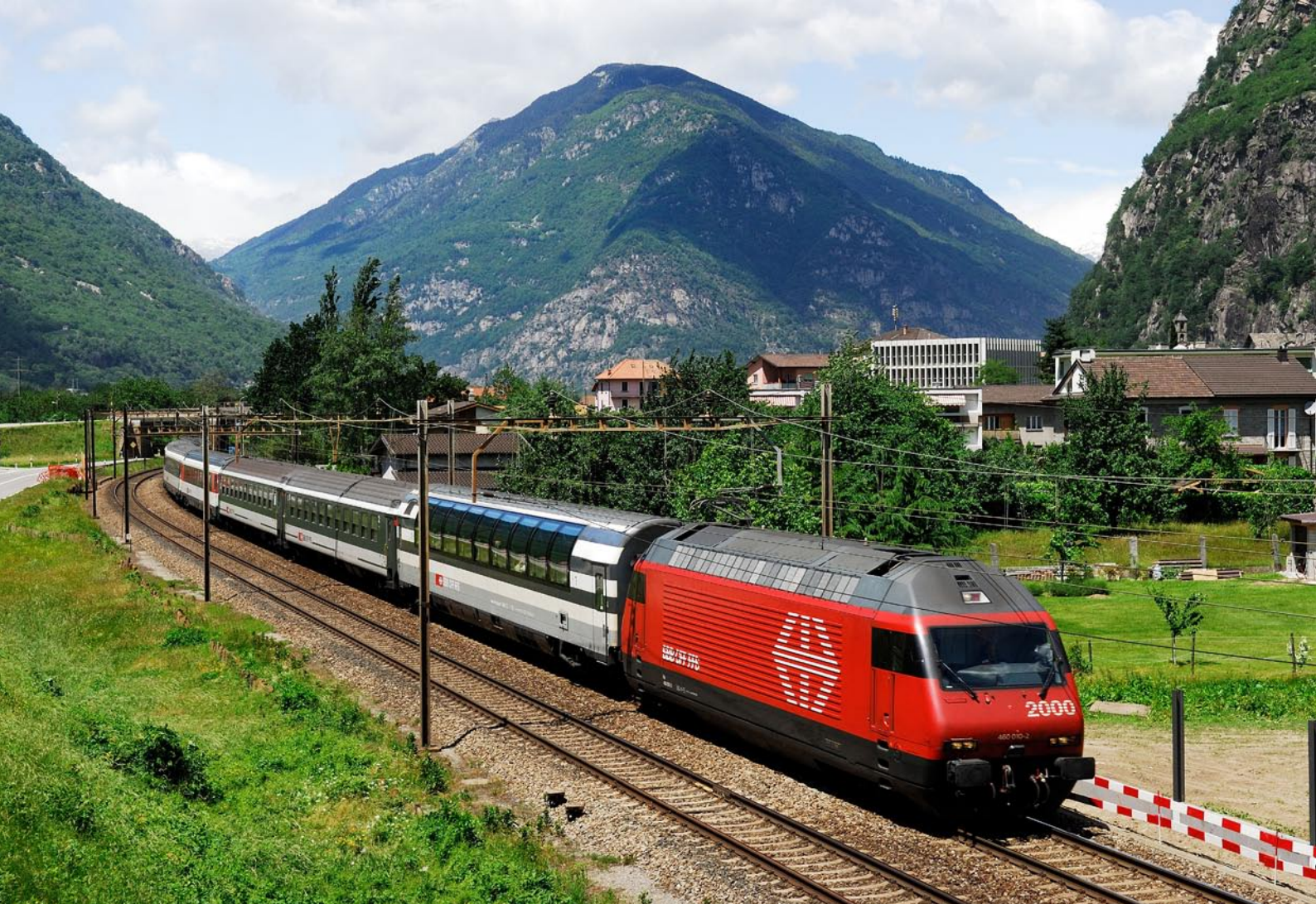
Above: Swiss Railways SBB Class 460 Bo-Bo No. 460 010-2 passes Osogna with train No. 2169, the 10.04 from Basel SBB to Locarno 'Wilhelm Tell Express' on 30 May 2006. Note the SBB observation carriage behind the loco. A fleet of 119 Class Re460 locos are in operation with SBB, introduced from 1992, these 8,180hp locos are also known as 'Lok 2000'. Brian Stephenson
