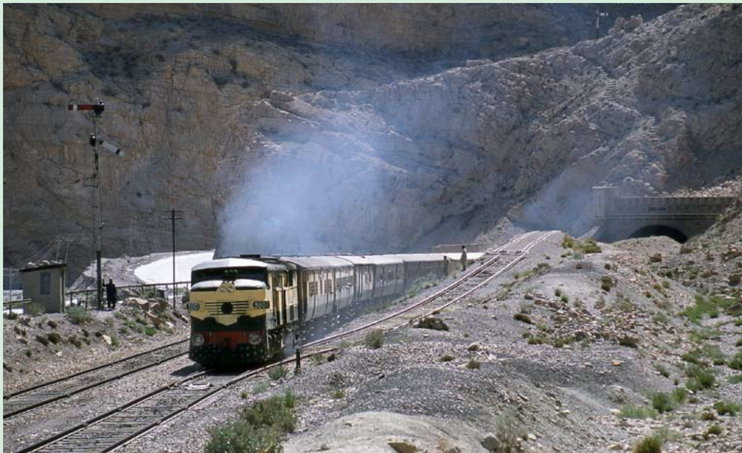
Above: With exhaust in true Alco style, late 1950s built Class ARPW20 (Model DL500C) No. 3801 is seen in Pakistan on the 1:25 Bolan Pass Grade at Dozan while powering the 'Sind Express' from Karachi to Quetta on 3 February 2001. A total of 42 of these Co-Co diesel-electric locos are in service, having been extensively rebuilt from the original Alco product. Note the semaphore signal high on the hill! Philip Cotterill Photographic details: Camera: Pentax K1000, Lens: Pentax, Film: Fujii Sensia 100ASA, Exposure: 1/250sec @ F11. Slide scanned on Epson4870 at 800dpi
